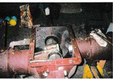
Each cylinder is cast integrally with one of the crankcase halves.
