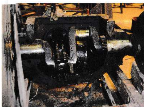
The crankcase isn't very big because the engine was not designed to have any oil standing in it.
